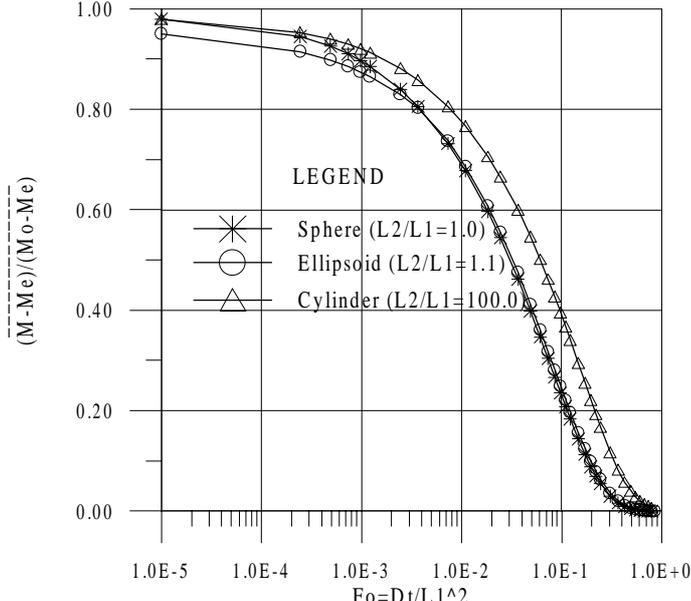
Figure 6 - Average concentration as a function of Fourier number, comparison between sphere, cylinder and ellipsoid.
