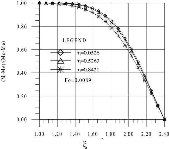
Figure 3- Profile of moisture content inside the prolate spheroid as a function of  $\xi$ ,  $L_2/L_1=1.1$
