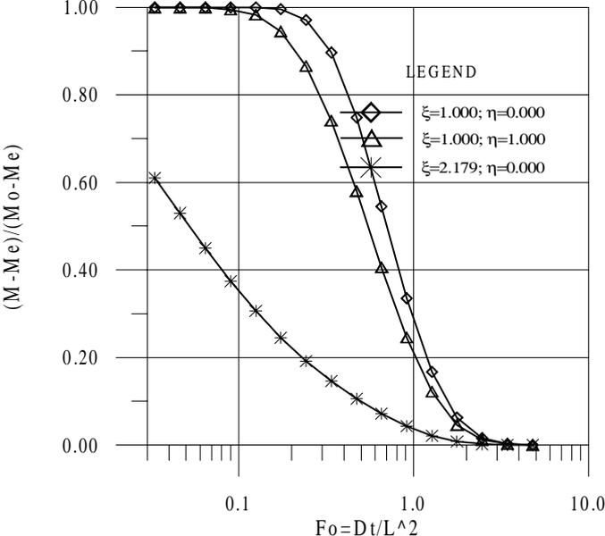
Figure 5- Moisture content in the center, focal point and near the surface for various  $Fo$ ,  $L_2/L_1=1.1$
