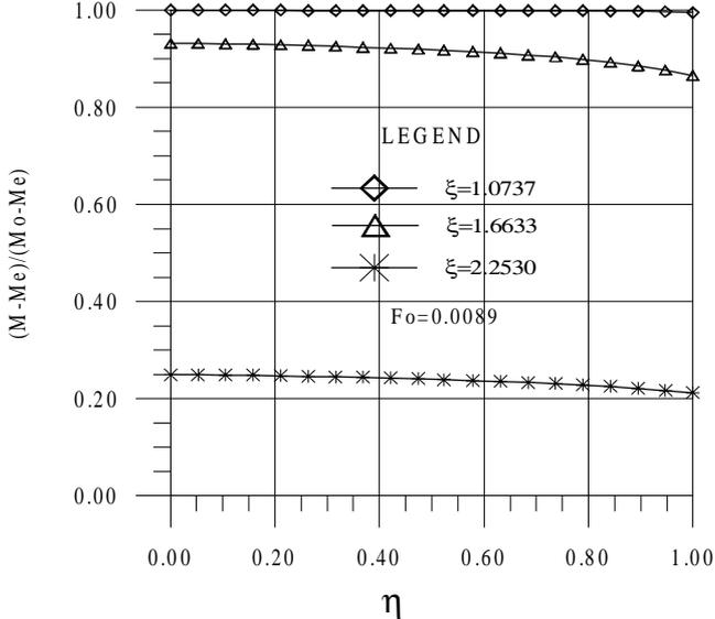
Figure 4- Profile of moisture content inside the prolate spheroid as a function of  $\eta$  ( $L_2/L_1=1.1$ )
