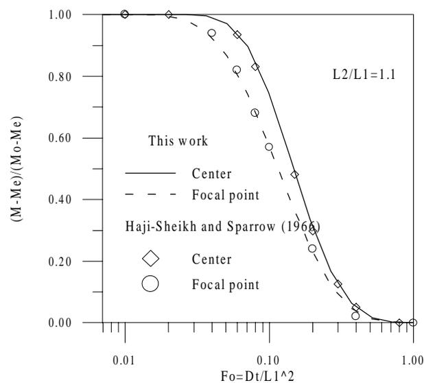
Figure 2 - Comparison between the moisture content ratio in the center and focal point of a spheroid with  $L_2/L_1=1.1$ , given by the authors and Haji-Sheikh & Sparrow (1966)
